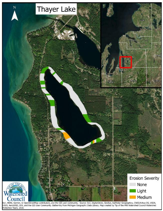
Figure 10 Erosion severity around Thayer Lake shoreline
